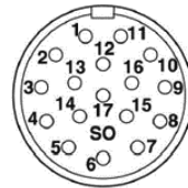
Pin assignment for female plug with external thread, 19-pin View of connection side
